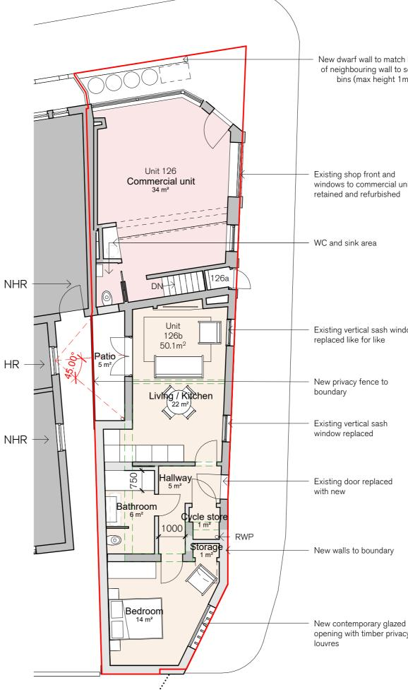
New dwarf wall to match height of neighbouring wall to screen bins (max height 1m)
